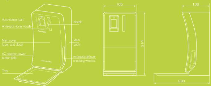
Name and structure Pure Hygiene PH-01/PH-02 (automatic door, air towel KTM series compatible)
